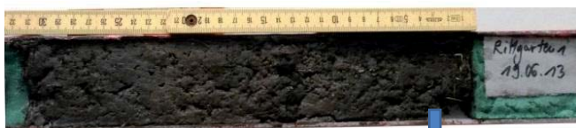
Fig. 2: Sediment core (Rittgarten) halved and sliced for further analysis.
