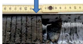
Fig. 2: Sediment core (Rittgarten) halved and sliced for further analysis.
