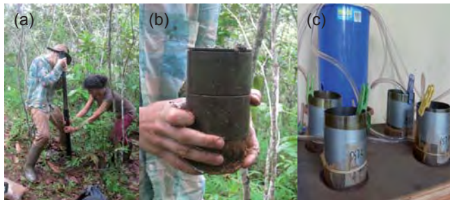
Fig. 1: Process of sample extraction: (a) withdrawing a sample from the soil, (b) extracting an undisturbed soil core, (c) measuring the water flux through a saturated soil sample
