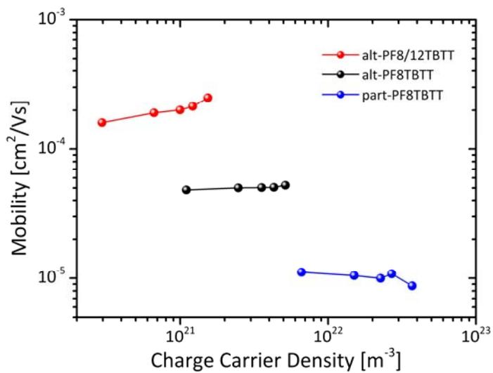
**S7.** Charge carrier density-dependence of the electron mobility for the three copolymers investigated here, extracted from intensity modulated Photo-CELIV experiments. Again, measurements were performed with a very short delay of 0.5  $\mu$ s.
