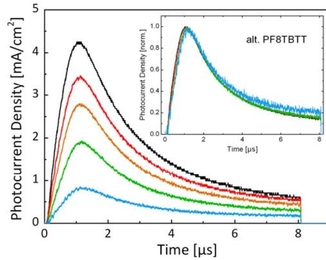
**S6.** Room temperature photo-CELIV transients at various excitation intensities measured for an alt-PF8TBTT CGL device. The capacitive loading current  $j_{\text{cap}}$  was subtracted to visualize photocurrents only. The inset shows normalized transients to demonstrate the intensity-independent shape of the photocurrents.
