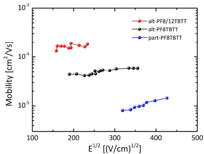
**S3.** Field-dependence of the electron mobility for the three copolymers investigated here, determined with Photo-CELIV. The devices were the same as described in the main text and measurements were performed with a short delay time of 0.5  $\mu$ s. A weak field-dependence is observed only for part-PF8TBTT.
