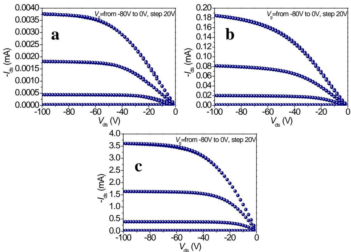
**Supplementary Figure S1. In-situ evolution of output characteristics of P3HT/PS (5% P3HT).** (a) As prepared. (b) and (c), After 33min and 1143 min in  $N_2$  atmosphere ( $O_2 \sim 1$  ppm and  $H_2O \sim 1$  ppm), respectively.
