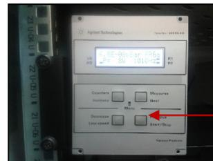
Step 1.6. Turbomolecular pump and pressure gauge controller.
