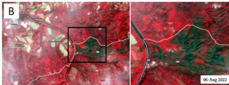
Figure 1. False color representation shows burned areas (green-black) in parts of Saxon-Bohemian Sandstone area, intact vegetation is shown in red colors. Source: ESA Sentinel-2, DaVis / BBK.
