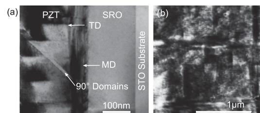
FIG. 1. TEM and AFM images of the PZT-SRO double layer grown onto an STO substrate by PLD. (a) The cross section TEM micrograph reveals that a minority of  $90^\circ$   $a$ -domains are embedded in the matrix of the  $c$ -axis grown tetragonal PZT film, as proved by the AFM topography image in (b) as well. Misfit dislocations (MD) and threading dislocations (TD) formed at the SRO-PZT interface and across the PZT film account for the lateral inhomogeneity on a sub-100 nm length scale.
