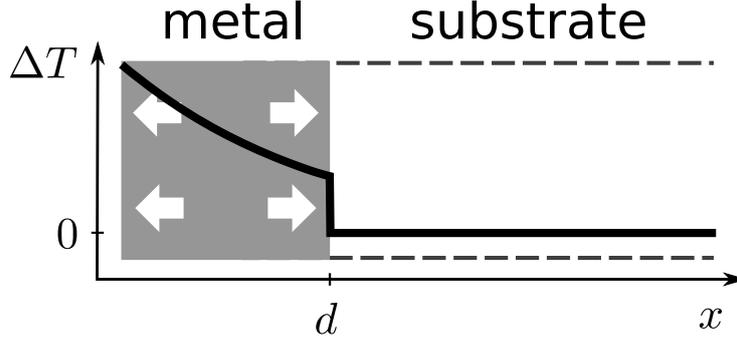
Figure 2.3: Schematic picture of a metal film with thickness  $d$  grown on top a substrate. The black line depicts the profile of the temperature change directly after photoexcitation. The white arrows symbolize that the metal wants to expand into the new equilibrium position.
