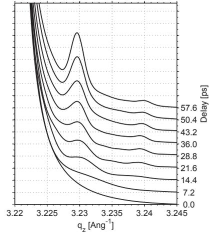
Figure 7: The side bands of the STO substrate Bragg peak are plotted for different pump-probe delays as waterfall diagram. The rise of the 1st order side band at  $q_z = 3.229 \text{ \AA}^{-1}$  and even a second order at  $q_z = 3.240 \text{ \AA}^{-1}$  of the excited phonon wave packet becomes stronger after each pump event.
