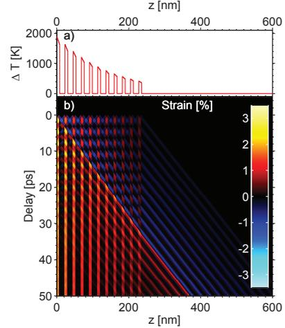
Figure 3: (Color online) a) Temperature change in the SL after excitation at  $t = 0$ . b) Spatio-temporal strain profile due to optical excitation of the SL film. The SL/Substrate interface is at  $z = 235 \text{ nm}$ .
