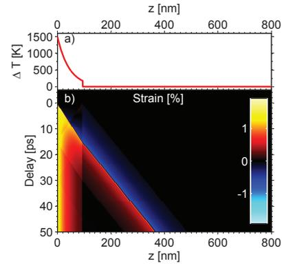
Figure 1: (Color online) a) Temperature change in the SRO thin film after excitation at  $t = 0$ . b) Spatio-temporal strain profile due to optical excitation of the SRO film. The SRO/STO interface is at  $z = 95 \text{ nm}$ .
