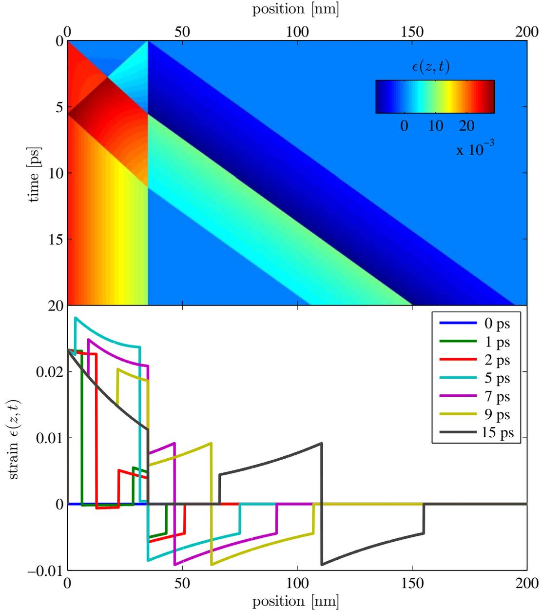
Figure 2.4: Shows the calculated strain evolution of a photo-excited SrRuO<sub>3</sub> film with thickness  $d = 35$  nm grown on the dielectric substrate SrTiO<sub>3</sub>.
