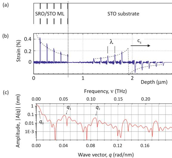
FIG. 1. (Color online) (a) Sketch of the five-period epitaxial SrRuO<sub>3</sub>/SrTiO<sub>3</sub> multilayer on top of the SrTiO<sub>3</sub> substrate. (b) Calculated strain profile in the sample along the surface normal, taken at 250 ps after the multilayer excitation. (c) Calculated spectrum of the strain pulse in the wave vector and frequency domains induced by the optical excitation. The vertical scale stands for the excitation fluence of 6 mJ/cm<sup>2</sup> used in the experiment.
