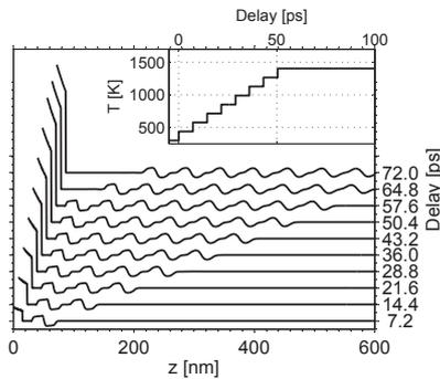
Figure 6: The strain profile for different pump-probe delays are plotted as waterfall diagram. For better visualization, the graphs are also shift along the  $x$ -axis. The amplitude of the thermal strain in the SRO layer has a maximum of approx. 1 % and the amplitude of the phonon wave packet is approx. 0.05 %. The inset shows the average temperature in the SRO layer due to the multipulse excitation of the sample.
