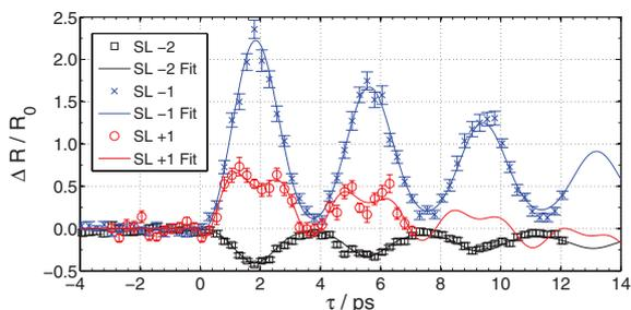
FIG. 5. (Color online) The rapid scanning technique was applied to measure the relative reflectivity  $\Delta R/R_0$  of the SL-2, SL-1, and SL+1 Bragg peaks of the LSMO/BST SL. The data for each SL peak was accumulated within  $\sim 20$  min per curve averaging over 40 complete delay scans with a frame rate of 2 Hz.
