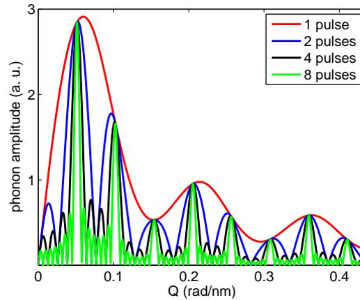
Fig. 1. **Calculated phonon spectra.** Spectral phonon amplitude present in the STO substrate after excitation of a 35 nm LSMO transducer by 1, 2, 4 and 8 pulses with a pulse spacing of  $\Delta T = 15.4$  ps. All pulse sequences have the same integrated pulse energy.
