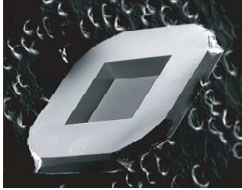
Figure 2.2: Photograph of a SiN membrane of dimensions 1\text{ mm} \times 1\text{ mm} \times 50\text{ nm} on a silicon chip (right panel from reference [17]).
