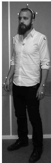
Figure 4: Each subject wears markers on hands, wrists, elbows, shoulders, sternum, and three markers mounted on a head-worn tiara.
