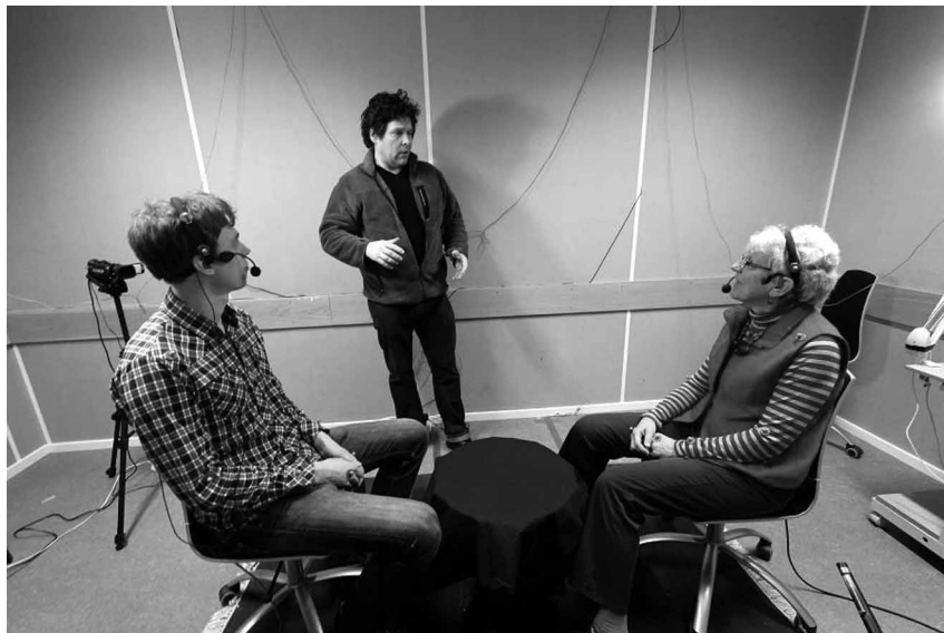
Figure 2: The recording studio during the instruction phase of a session. Subjects are wearing headmounted microphones and head bands with Optitrack markers, and additional markers are fixed to torsos, arms and hands (Edlund and Beskow 2010).
