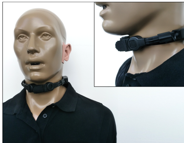
Figure 1. Throat microphone attached to a dummy head.
