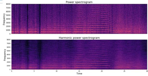
Due to changing the sampling rate frequency; the original frequency content is equal to: The frequency we see in the axis/16.
