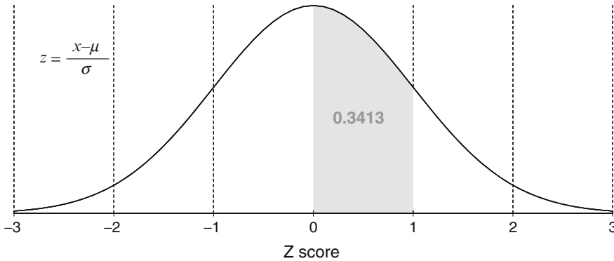
Fig. 2.3 Z-score and the corresponding cumulative probability and percentile (proportion). For normal distribution, the Z-score of 0 divides the total area into two equal halves. Thus, the Z-score of 1 corresponds to the 84th percentile ( =0.5 + 0.34 ), i.e., 84% of the population are measured lower than z-score of 1. A Z-score is calculated as dividing the difference between measured value ( x ) and the mean ( \mu ) by standard deviation ( \sigma )
