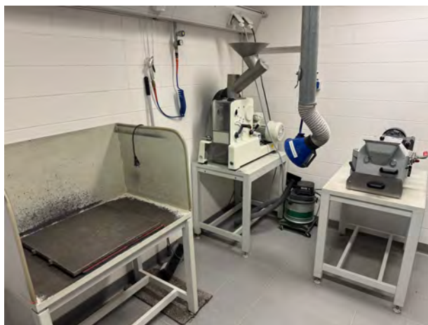
Figure 1.1 – Panoramic view of room 0.41, showing (from left to right) the hammer plate, jaw crusher, and disk mill.
